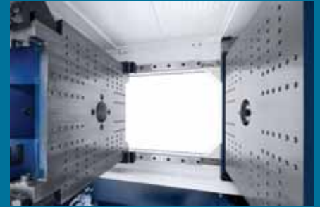
Side walls become tie bars and as a result enlarge the mold platen dimension by 70%.
