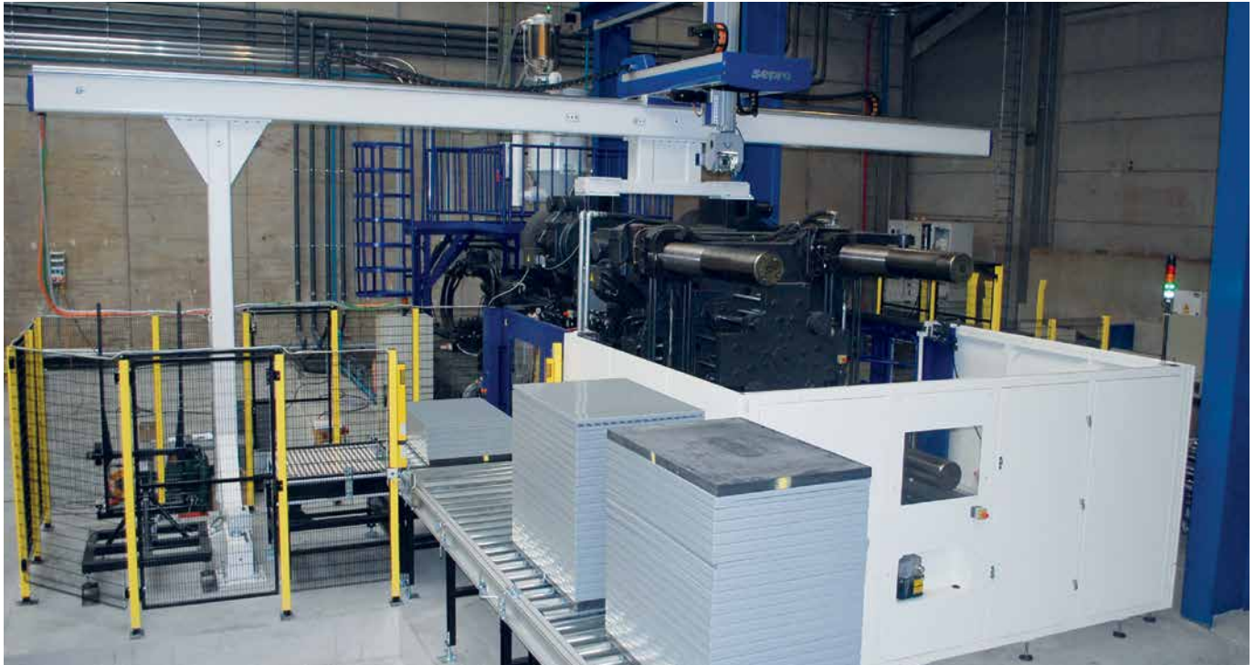
Since this Summer, a Jupiter 18,500 II machine is Integrated in a fully-automatic production cell, the panels are extracted, planned with a optical quality control with a camera system and stacked individually back-to-back.
